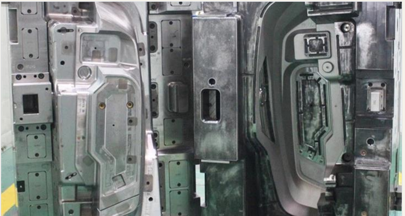
AUTOMOTIVE DOOR INJECTION MOULD • CORE / CAVITY TOOLING
